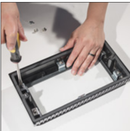
10. Remove glass lens and clips from lens frame and discard.
