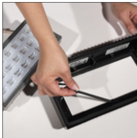
11. Remove existing black gasket from lens frame and clean surface. New optic assembly will include a gasket.
