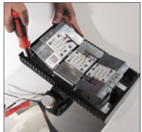
3. Loosen and remove screws securing LED assembly. Set screws aside.
