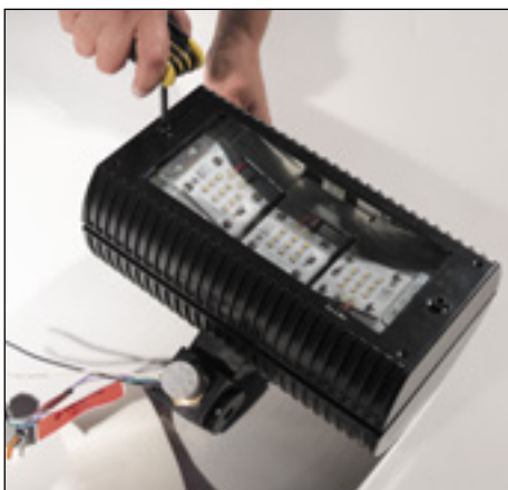
1. Loosen (2) 1/4"-20 hex socket bolts with 3/16" hex key and discard bolts.
