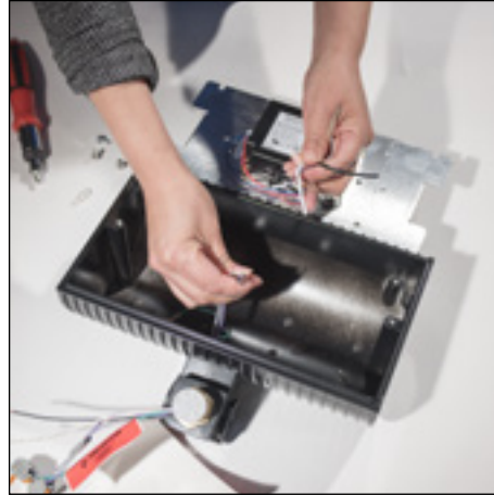
5. Remove wire nuts and disconnect LED assembly wiring. Discard LED assembly.
